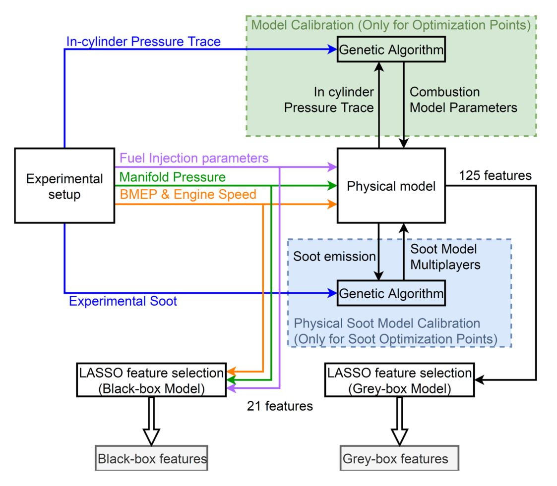
Figure 3: Diesel soot emission modeling process using grey-box techniques
