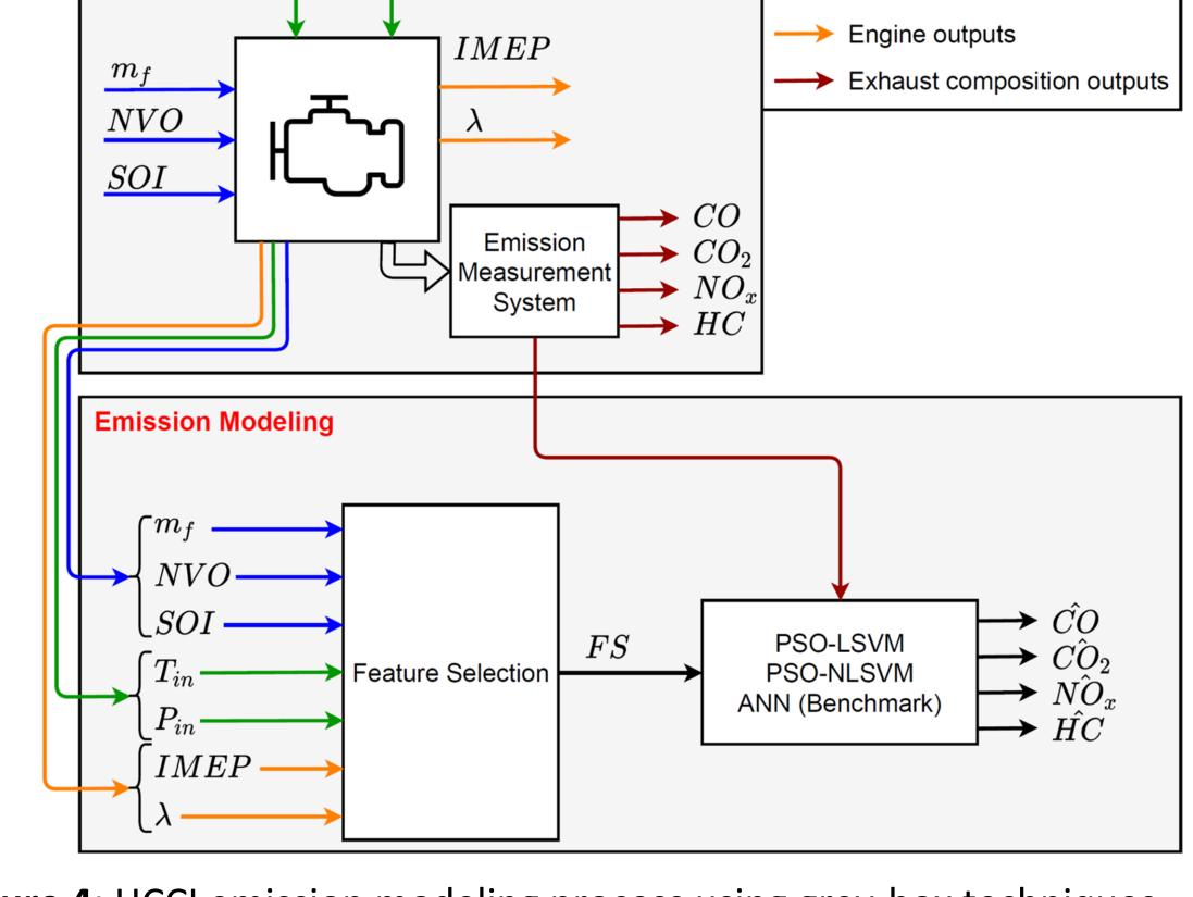
Figure 4: HCCI emission modeling process using grey-box techniques
