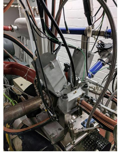
Figure 2: HCCI experimental setup
