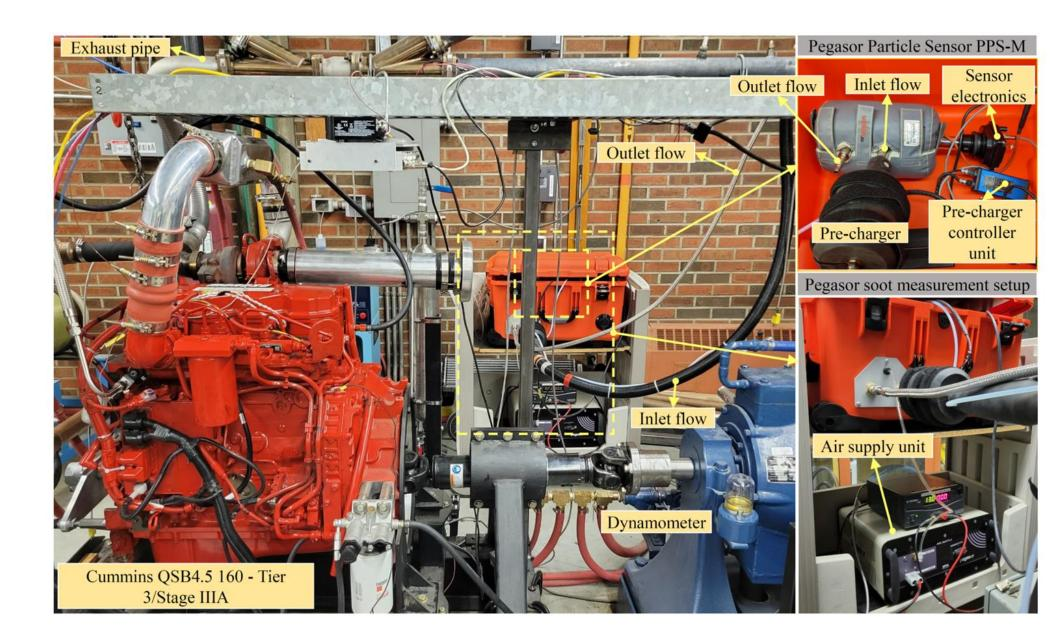
Figure 1: Diesel experimental setup
